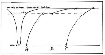
Fig 6 Routes to Interplanetary Destinations –A is totally reusable to GEO, B is GEO to Interplanetary via Lightweight Craft Assembled at Gateway, C is the SLS/Orion-type approach.
