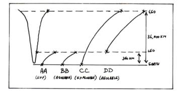
Fig App 1 Comparison cases for various ways of getting crews or cargo out of Earth's gravity well and up to GEO
