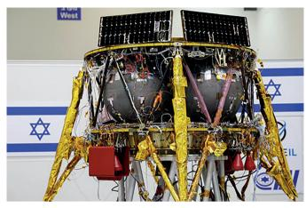
▲ Images of the SpaceIL lunar lander/hopper. An early concept (left) and the flight model prior to its planned February 2019 launch.
