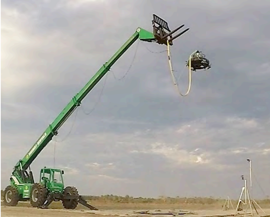
Fig 5 Demonstration of a lander/hopper (suspended and hovering from test rig) at their KSC test facility, in December 2014, by the former GLXP Team MoonExpress, USA.
